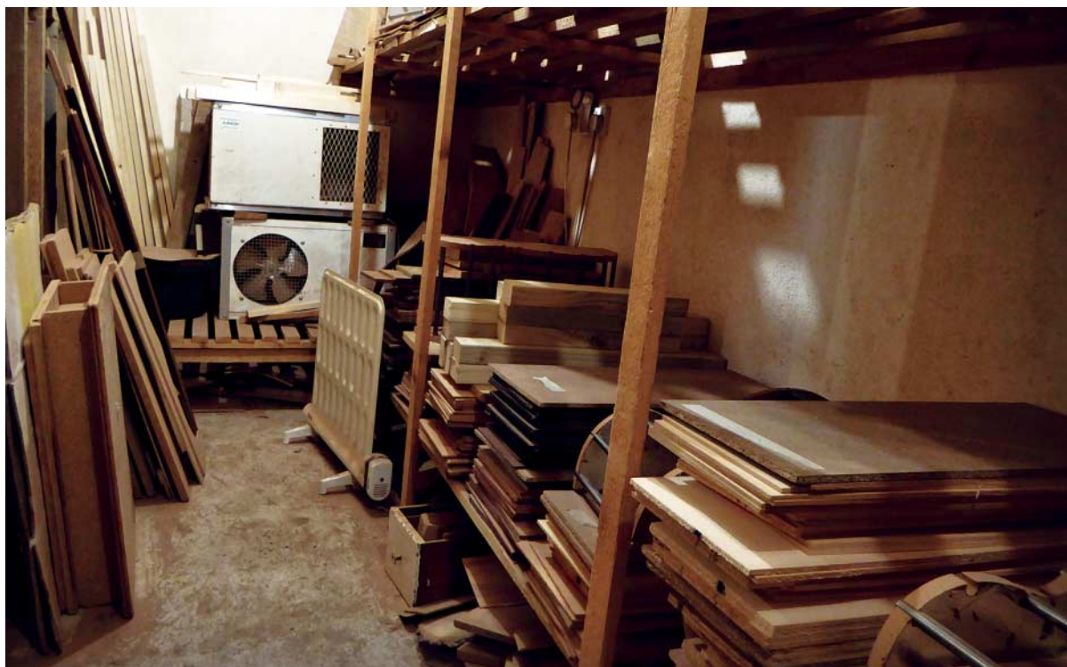
The drying room – one of the most important rooms at the Brook workshop, where all wood components of guitars are acclimatised together before assembly, to ensure consistent moisture content.
